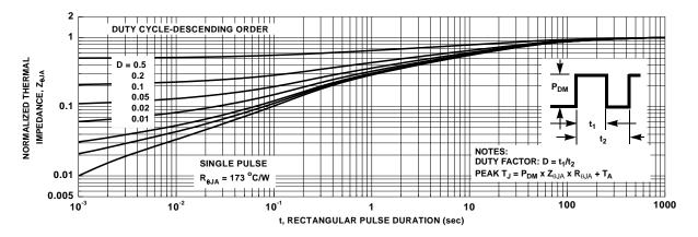
Figure 12. Junction-to-Ambient Transient Thermal Response Curve
