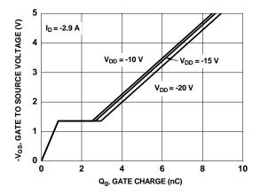
Figure 7. Gate Charge Characteristics
