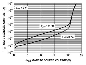
Figure 9. Gate Leakage vs Gate to Source Voltage
