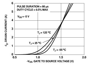
Figure 5. Transfer Characteristics
