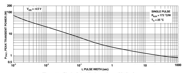
Figure 11. Single Pulse Maximum Power Dissipation
